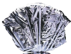
▲ Figure 7.22 Elemental silicon. Silicon is an example of a metalloid. Although it looks metallic, silicon is brittle and is a poor thermal and electrical conductor as compared to metals. Large crystals of silicon are sliced into thin wafers for use in integrated circuits.
