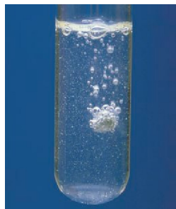
▲ Figure 7.29 Elemental calcium solution. Calcium metal reacts with water to form hydrogen gas and aqueous calcium hydroxide, \text{Ca}(\text{OH})_2(\text{aq}) .
