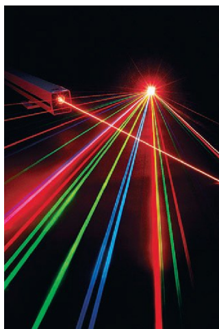
▲ Figure 6.10 Monochromatic radiation. Lasers produce light of a single wavelength, which we call monochromatic light . Different lasers produce light of different wavelengths. The photo shows beams from a variety of lasers that produce visible light of different colors. Other lasers produce light that is not visible, including infrared and ultraviolet light.
