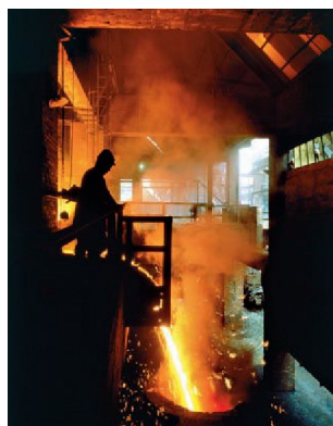
▲ Figure 6.6 Color as a function of temperature. The color and intensity of the light emitted by a hot object depend on the temperature of the object. The temperature is highest at the center of this pour of molten steel. As a result, the light emitted from the center is most intense and of shortest wavelength.
