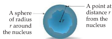
▲ Figure 6.21 Probability at a point. The probability density, \psi(r)^2 , gives the probability that the electron will be found at a specific point at distance r from the nucleus. The radial probability function, 4\pi r^2 \psi(r)^2 , gives the probability that the electron will be found at any point distance r from the nucleus—in other words, at any point on the sphere of radius r .
