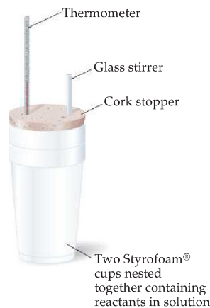
▲ Figure 5.17 Coffee-cup calorimeter. This simple apparatus is used to measure heat-accompanying reactions at constant pressure.
