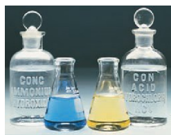
▲ Figure 4.7 The acid–base indicator bromthymol blue. The indicator is blue in basic solution and yellow in acidic solution. The left flask shows the indicator in the presence of a base, aqueous ammonia (labeled as ammonium hydroxide). The right flask shows the indicator in the presence of hydrochloric acid, HCl.
