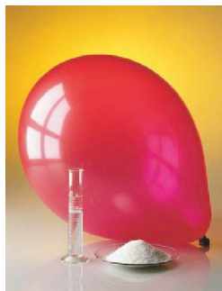
▲ Figure 3.9 One mole each of a solid, a liquid, and a gas. One mole of NaCl, the solid, has a mass of 58.45 g. One mole of H 2 O, the liquid, has a mass of 18.0 g and occupies a volume of 18.0 mL. One mole of O 2 , the gas, has a mass of 32.0 g and occupies a balloon whose diameter is 35 cm.
