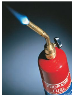
▲ Figure 3.7 Propane burning in air. The liquid propane, C 3 H 8 , vaporizes and mixes with air as it escapes through the nozzle. The combustion reaction of C 3 H 8 and O 2 produces a blue flame.
