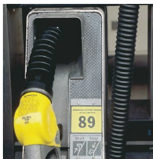
▲ Figure 25.8 Octane rating. The octane rating of gasoline measures its resistance to knocking when burned in an engine. The octane rating of this gasoline is 89, as shown on the face of the pump.
