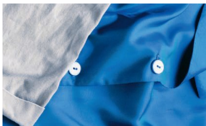
▲ Figure 25.18 Cellulose acetate fiber. The blue garment, woven from cellulose acetate fiber, has a silky, vibrant texture compared with the white garment, woven from simple cotton fiber.
