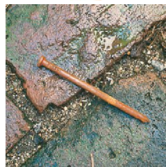
▲ Figure 19.2 A spontaneous process. Elemental iron in the shiny nail in the top photograph spontaneously combines with \text{H}_2\text{O} and \text{O}_2 in the surrounding air to form a layer of rust— \text{Fe}_2\text{O}_3 —on the nail surface.
