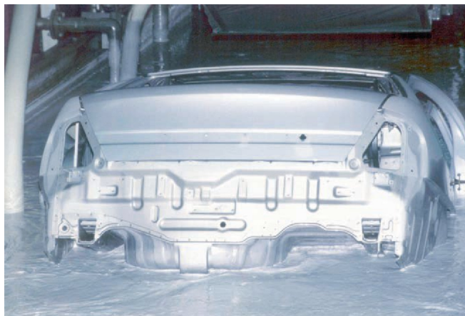
▲ Figure 18.23 Green chemistry for your car. An automobile body receives a corrosion-protection coating containing yttrium in place of lead.
