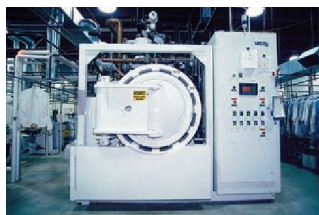
▲ Figure 18.22 Green chemistry for your clothes. This dry-cleaning apparatus employs liquid \text{CO}_2 as the solvent.
