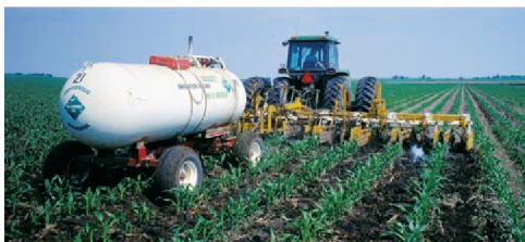
▲ Figure 15.5 Liquid ammonia used as fertilizer. Ammonia, produced by the Haber process, can be added directly to the soil as a fertilizer. Agricultural use is the largest single application of manufactured NH_3 .
