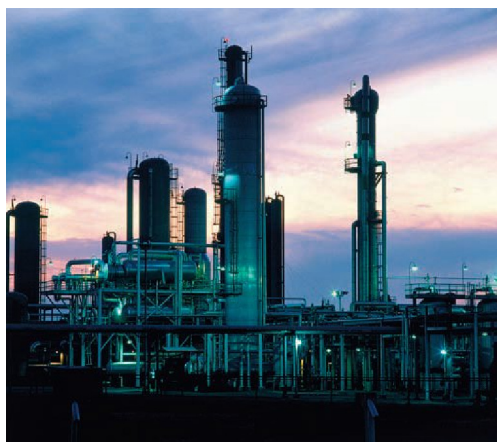
▲ Figure 13.21 Separating volatile components. In an industrial distillation tower, such as the ones shown here, the components of a volatile organic mixture are separated according to boiling-point range.
