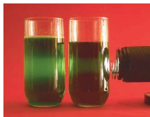
▲ Figure 13.26 Tyndall effect in the laboratory. The glass on the left contains a colloidal suspension; that on the right contains a solution. The path of the beam through the colloidal suspension is visible because the light is scattered by the colloidal particles. Light is not scattered by the individual solute molecules in the solution.
