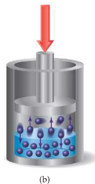
▲ Figure 13.14 Effect of pressure on gas solubility. When the pressure is increased, as in (b), the rate at which gas molecules enter the solution increases. The concentration of solute molecules at equilibrium increases in proportion to the pressure.
