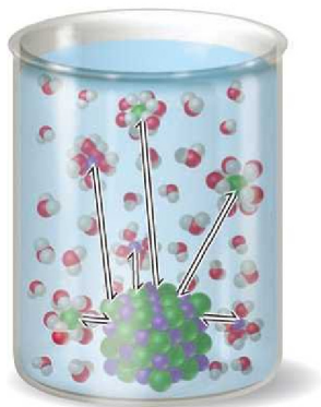
▲ Figure 13.9 Dynamic equilibrium in a saturated solution. In a solution in which excess ionic solute is present, ions on the surface of the solute are continuously passing into the solution as hydrated species, while hydrated ions from the solution are deposited on the surfaces of the solute. At equilibrium in a saturated solution, the two processes occur at equal rates.
