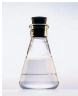
Hexane is insoluble in water. Hexane is the top layer because it is less dense than water.
