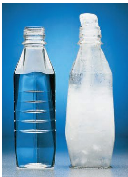
▲ Figure 11.11 Expansion of water upon freezing. Water is one of the few substances that expand upon freezing. The expansion is due to the open structure of ice relative to that of liquid water.
