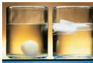
▲ Figure 11.9 Comparing densities of liquid and solid phases. As with most other substances, the solid phase of paraffin is denser than the liquid phase, and the solid therefore sinks below the surface of the liquid paraffin in the beaker on the left. In contrast, the solid phase of water, ice, is less dense than its liquid phase (right beaker), causing the ice to float on the water.
