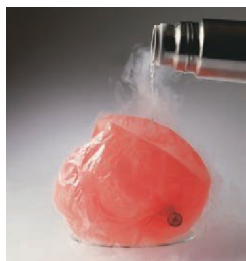
▲ Figure 10.8 An illustration of the effect of temperature on volume. As liquid nitrogen ( -196^\circ\text{C} ) is poured over a balloon, the gas in the balloon is cooled and its volume decreases.
